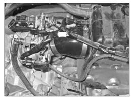
9. Reconnect the fuel injection electrical connections.
