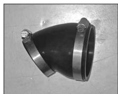
7. Install the provided hose clamps onto the K&N® silicone hose (084096) as shown.
