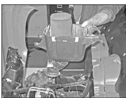
17. Remove the lower air box from the vehicle as
