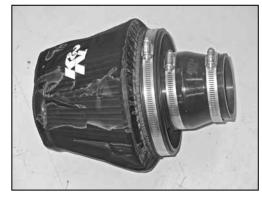
24. Install the K&N® Drycharger® onto the air filter as shown.
