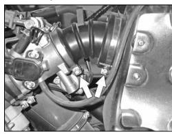
5. Loosen the two hose clamps which secure the stock intake hose to the throttle body and air chamber.
