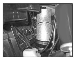
25. Install the K&N® intake tube into the silicone hose and align with the tube mounting bracket installed onto the heat shield, then secure the intake tube with the hose clamp and hardware provided.
