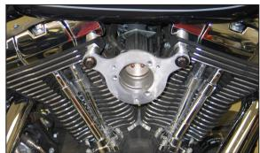
10. Using the two provided crankcase breather bolts; install the back plate onto the vehicle as shown. Do not tighten the breather bolts at this time.
