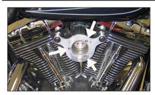
11. Install the provided gasket between the throttle body and back plate and then secure the back plate to the throttle body with the hardware provided. Tighten the crankcase breather bolts.
