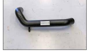
21. Install the provided vent fitting into the  $K\&N^{\circledast}$  intake tube.
