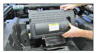
5. Loosen and remove the two hose clamps that secure the fresh air and clean air ducts to the air filter housing. Remove the air filter housing from the vehicle.
