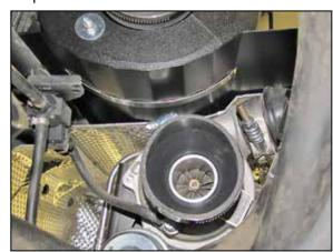
19. Install the provided coupler hose (08667) onto the turbo inlet and secure with the provided hose clamp.
