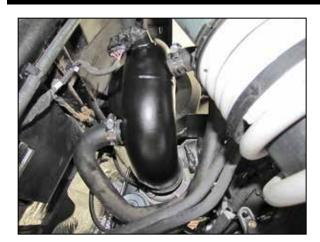
22. Install the K&N® intake tube into the coupling hoses, align for best fit and then secure with the provided hose clamps. Reconnect the inlet temperature sensor electrical connection and connect the BOV hose and crank case breather hoses. Secure the hoses with the provided hose clamps.
