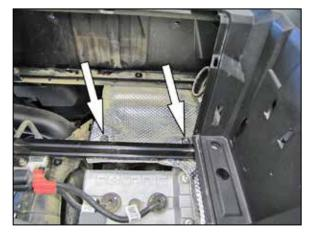
9. Remove the two nuts and bolts shown that secure the heat shielding to the chassis. NOTE: On some models there may be a lip on the drivers side of the heat shield which will need to be folded flat.
