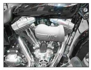
11. Install the K&N $^{\! \rm B}$  intake tube with the gasket and provided hardware.
