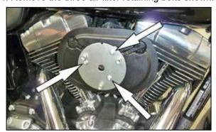
5. Remove the three retaining bolts for the air filter adapter as shown.
