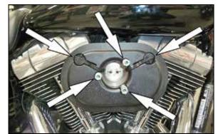
6. Remove the two breather caps and two breather bolts under caps then remove the three base retaining bolts as shown.
