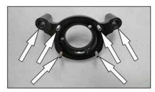
9. Install the remaining two o rings onto the front of the back plate as shown. Install the four provided studs with thread locker positioned into the back plate.
