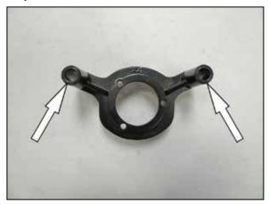
8. Install two of the o rings provided onto the back side of the K&N® back plate as shown.
