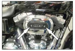
2. Remove the two screws that attach the number plate.
