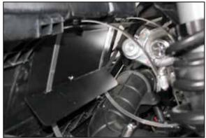
18. Install the air filter mount into the vehicle so that the hose clamp adjusters are on the top and the bolts are off set to the left. Secure the mount with the hardware provided.
