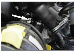
12. Loosen the hose clamp securing the intake flex hose to the air box.
