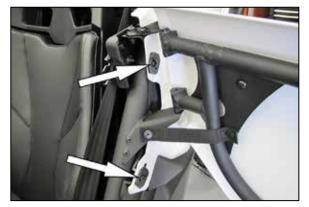
6. Open the door and remove the two fasteners securing the front of the fender.
