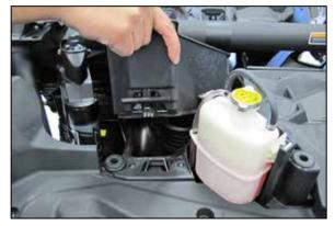
9. Lift and remove the clutch filter.
