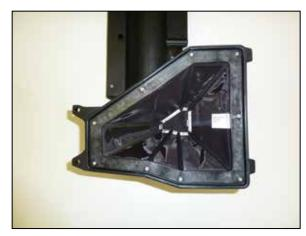
7. Install the dry charger assembly into the K&N® fresh air intake system and secure with the provided hardware.
