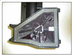
8. Install the provided gasket onto the lower portion of the factory fresh air housing and then install the K&N® fresh air system and secure with the hardware provided.
