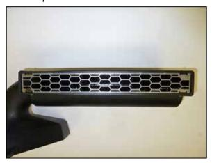
9. Install the inlet mesh into the K&N® fresh air intake and secure with the provided hardware.
