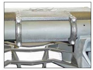
11. Secure the K&N® fresh air system to the chassis bar with the provided clamps and hardware.
