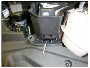
3. Release the locking clip and remove the factory dust filter.
