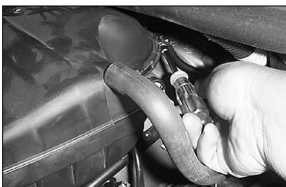
2. Loosen the hose clamp on the air cleaner at the throttle body.
