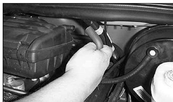
3. Disconnect the crankcase vent line from the air cleaner.
