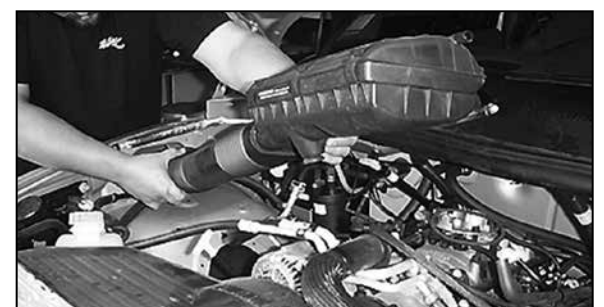
5. Detach the air inlet duct from the inner fender and remove the entire air cleaner assembly. NOTE: Remove the OE gasket as it will not be used. NOTE: K&N Engineering, Inc., recommends that customers do not discard factory air intake.
