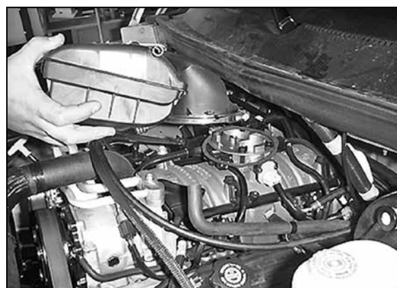
4. Pull firmly upwards to remove the air cleaner away from the throttle body.
