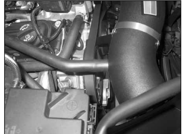
21. Connect the crankcase vent hose to the intake tube.
