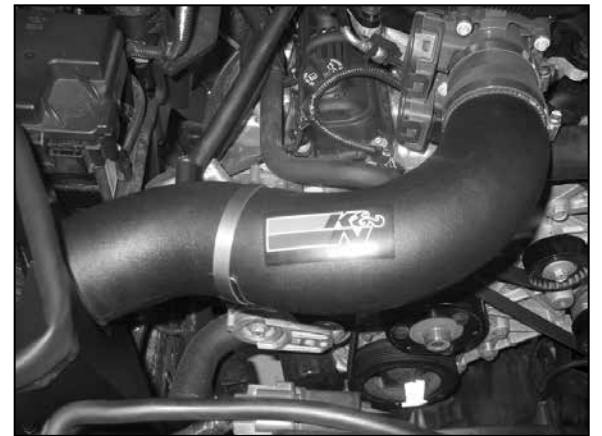
20. Insert the intake tube into the silicone hose at the throttle body and align with the mounting bracket installed in step #12 and then secure with the hose clamps provided.
