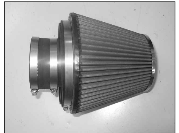
23. Install the silicone hose (08630) onto the air filter adapter and secure with the provided hose clamp.
