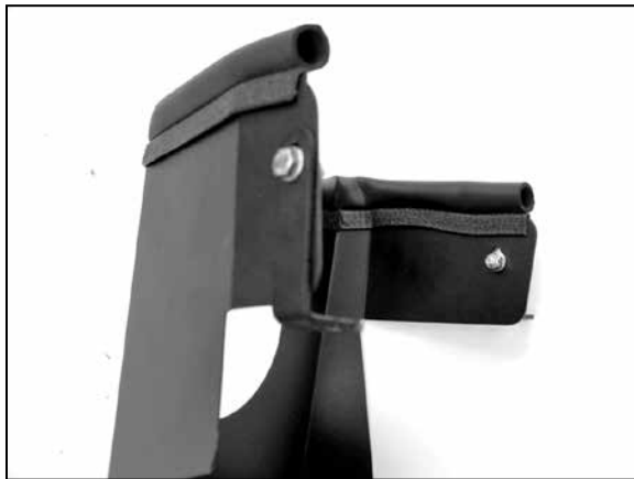
18. Install the supplied "L" bracket (07195) onto the heat shield as shown with the provided hardware.
