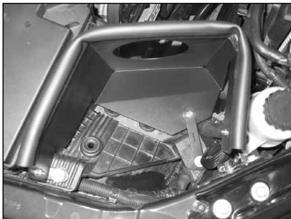
19. Install the heat shield assembly into the engine compartment and secure with the three bolts removed in step #12.
