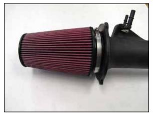
14. Install the air filter onto the end of the K&N<sup>®</sup> intake tube and secure with the provided hose clamp.
