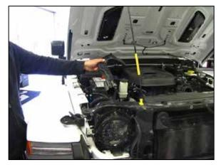
8. Remove the two bolts that secure the fresh air duct to the core support and then remove the duct from the vehicle.
