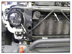
7. Remove the two bolts securing the diagonal core support brace and remove the brace. **NOTE: This brace will be reinstalled.**
