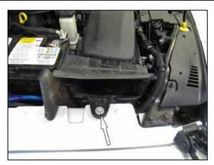
5. Remove the bolt that secures the fresh air duct to the fender. Remove the complete intake system
