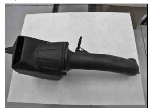
15. Install the intake tube assembly into the  $K\&N^{\mbox{\tiny \$}}$
