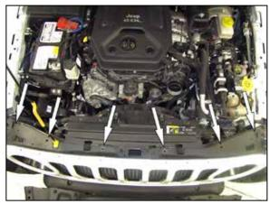
6. Remove the six retaining clips that secure the grill assembly to the core support. Remove the grill assembly.
