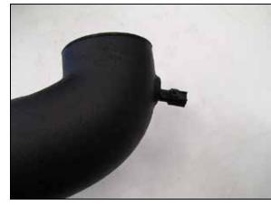
13. Remove the inlet air temperature sensor from the factory intake tube. Remove the O-ring from the sensor and then install the sensor into the K&N<sup>®</sup> intake tube using the provided grommet.
