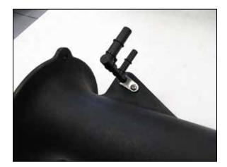
12. Install the O-ring onto the ejector fitting provided and then install the fitting into the K&N<sup>®</sup> intake tube. Secure the fitting with the clip and hardware provided.
