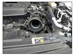
16. Install the provided step coupler onto the throttle body and secure with the provided hose clamp.
