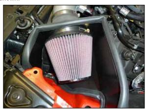
19. Install the K&N® air filter onto the filter adapter and secure with the provided hose clamp.
