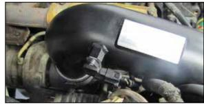
22. Reconnect the inlet air temperature sensor electrical connection.
