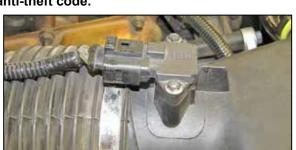
2. Disconnect the inlet air temperature sensor electrical connection.
