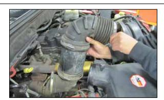
4. Remove the intake hose from the vehicle.
