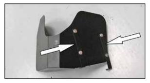
8. Install the two provided heat shield mounting brackets (07159) onto the heat shield as shown using the provided hardware.
