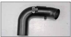
18. Install the inlet air temperature sensor into the K&N® intake tube as shown.
