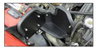
15. Install the heat shield assembly onto the inserted nuts then secures it to the fan shroud and inserted nuts with the provided hardware.
