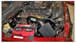
23. Reconnect the vehicle's negative battery cable. Double check to make sure everything is tight and properly positioned before starting the vehicle.
