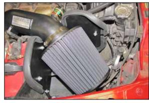
21. Install the K&N® air filter onto the K&N® intake
