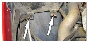
7. Remove the two air box mounting grommets from the mount.
