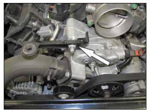
8. Remove the nut securing the factory intake resonator bracket to the engine and then remove the bracket from the engine.
