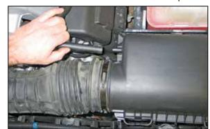
6. On models equipped with a 6.4L, disconnect the crank case vent from the air filter housing as shown.
