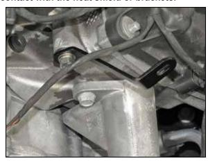
13. Install the tube mounting bracket (010088A) onto the cylinder head as shown. Be sure to place the provided spacer between the bracket and cylinder heads.
