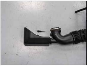
15. Remove the factory inlet air temperature sensor from the factory intake tube.
