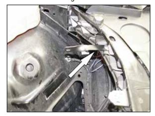
9. Install the heat shield mounting bracket (070772A) onto the core support using the provided hardware.
