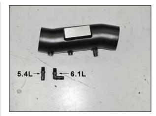
17. Install the appropriate 1/4npt fitting into the  $K\&N^{\odot}$  intake tube. The straight fitting is for 5.7L engines and the 90° fitting is for 6.0L.
