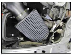
26. Install the K&N $^{\mbox{\tiny B}}$  air filter and secure with the provided hose clamp.
