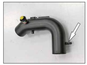
22. Install the 5/8 barb, 1/4npt crank case vent fitting provided into the  $K\&N^{\otimes}$  intake tube as shown.
