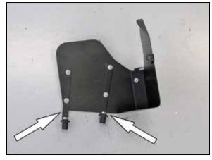
13. Install the heat shield mounting bracket assemblies (07159) onto the heat shield as shown using the provided hardware.
