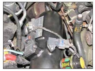
27. Reconnect the mass air sensor and inlet air temperature sensor electrical connections. **NOTE: The factory wiring harness may need to be adjusted so that the harness is not too tight.**
