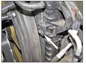
16. Remove the fan shroud bolt shown.
