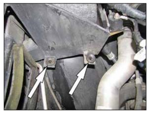
9. Remove the two air box mounting grommets shown.
