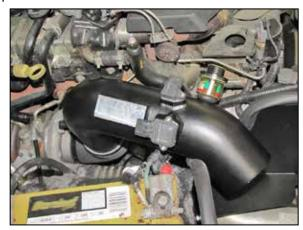
24. Install the K&N<sup>®</sup> intake tube assembly into the silicone hose at the turbo inlet and align with the mounting bracket installed on the heat shield. Secure the heat shield with the provided hardware and hose clamp.
