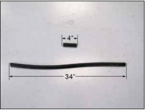
14. Cut the provided edge trim into two lengths. One length will be 34" long and one section will be 4" long.
