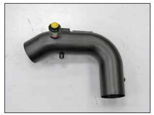
21. On vehicles equipped with a filter minder, install the factory grommet and filter minder into the K&N $^{\circ}$  intake tube as shown.
