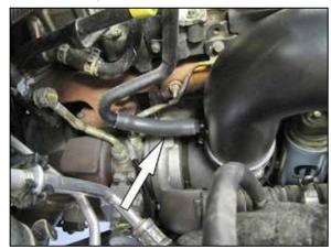
25. Install the provided crank case vent hose onto the fitting installed into the  $K\&N^{\mbox{\scriptsize \$}}$  intake tube and
