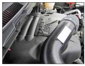
28. Choose the appropriate inlet air temperature sensor extension harness and then connect Install it too the inlet air temperature sensor and vehicle harness.
