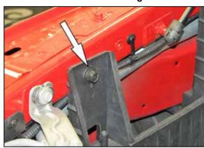
18. Remove the front air box mounting bracket bolt shown.
