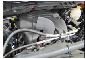
21. Install the provided silicone hose (08498) onto the throttle body and secure with the provided hose clamp.
