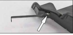
17. Install the heat shield mounting bracket (083103-1A) onto the heat shield using the provided hardware.
