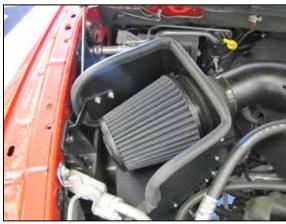
29. Install the K&N® air filter and secure with the provided hose clamp.
