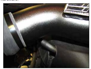
27. Connect the crank case vent hose to the fitting installed into the K&N<sup>®</sup> intake tube and secure with the provided hose clamp.
