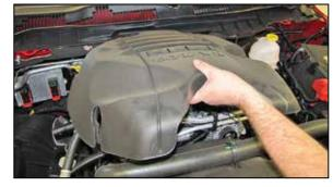
6. Lift up the engine cover and remove it from the vehicle.
