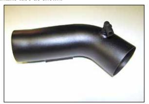
23. Install the vent fitting into the K&N® intake tube as shown.
