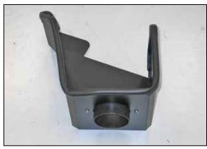
14. Install the provided filter adapter into the K&N<sup>®</sup> heat shield and secure with the provided hardware.
