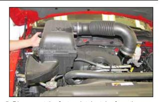
5. Disconnect the factory intake tube from the throttle body, then lift up the intake assembly and remove it from the vehicle.
