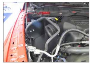
20. Install the heat shield into the vehicle and secure with the factory bolts from steps #18 and #10.
