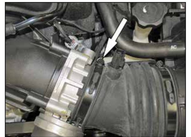
5. Loosen the hose clamp securing the intake tube to the throttle body.
