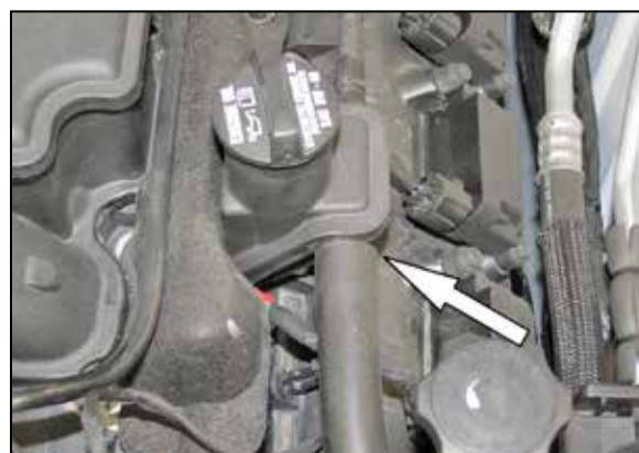
4. Disconnect the crank case vent hose from the valve cover.
