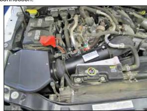
38. Reconnect the vehicle's negative battery cable. Double check to make sure everything is tight and properly positioned before starting the vehicle.
