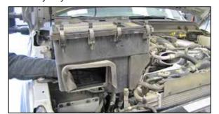
10. Remove the lower air box from the vehicle. NOTE: K&N Engineering, Inc., recommends that customers do not discard factory air intake.
