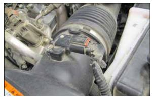
2. Release the red locking tab and then disconnect the mass air sensor electrical connection and unhook the wiring harness from the air box.
