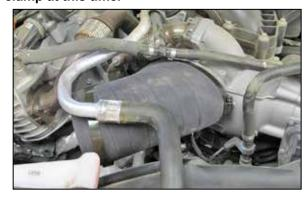
30. Install the silicone hose (08501) onto the turbo inlet as shown.
