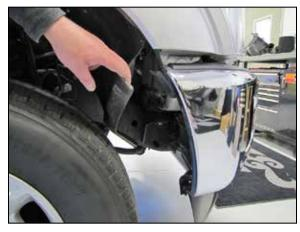
14. Remove the 5 bolts and one push pin securing the front of the inner fender panel and then pull the inner fender panel back to gain access to the bottom of the fresh air intake duct.
