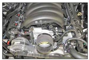
13. Install the provided coupling hose (08698 for 5.3L, 08497 for 6.2L) onto the throttle body and secure with the provided hose clamps.
