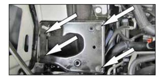
7. Remove the four bolts securing the air box mounting tray and then remove the tray from the vehicle.
