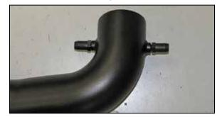
17. Install the two provided crank case vent fittings into the K&N $^{\odot}$  intake tube as shown.
