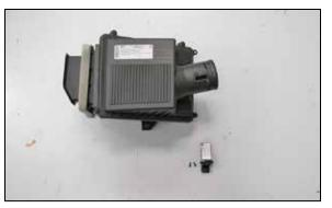
15. Remove the two screws securing the mass air sensor to the factory air box and then remove the sensor from the air box.
