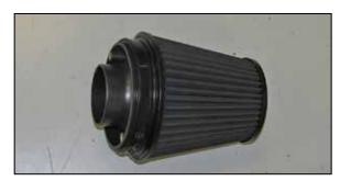
10. Install the filter adapter into the K&N<sup>®</sup> air filter and secure with the provided hose clamp.
