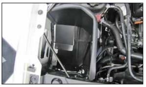
9. Install the heat shield assembly and secure to the air box mounting plate location using the three factory bolts from step #7.
