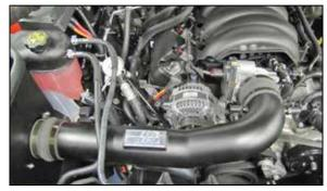
18. Install the K&N<sup>®</sup> intake tube into the hose at the filter adapter and then into the hose at the throttle body. Adjust the tube for proper fit and then secure with the provided hose clamps.
