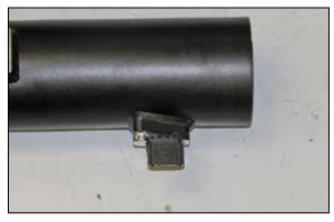
16. Install the mass air sensor into the K&N<sup>®</sup> intake tube and secure with the provided hardware.
