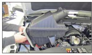
6. Pull up the air box to release it from the mounting grommets and then remove the factory air box from the vehicle.
