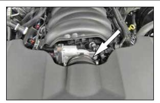
4. Loosen the two hose clamps securing the intake plenum to the factory air box and to the throttle body.
