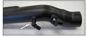
14. Install the 90° vent fitting into the K&N $^{\odot}$  intake tube as shown.
