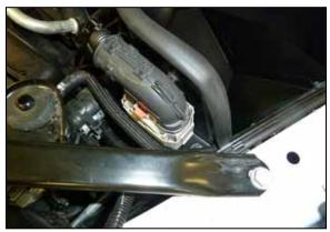
15. Connect the wiring bulk connector onto the bracket installed onto the heat shield.
