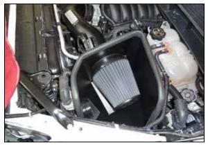
26. Install the K&N<sup>®</sup> air filter onto the adapter and secure with the provided hose clamp.
