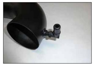
20. Install the provided 90° quick connect fitting into the K&N $^{\mbox{\tiny \$}}$  intake tube as shown.
