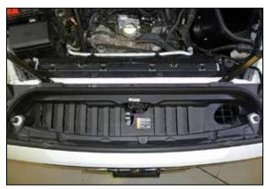
16. Reinstall the radiator valence and secure with the ten factory clips.
