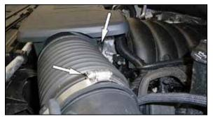
4. Loosen the hose clamps that secures the intake plenum to the air filter housing and to the throttle body. Disconnect the plenum connections at the air filter housing and then rotate the plenum counter clockwise to disengage the keyed mount and separate it from the throttle body. NOTE: The wiring harness anchored to the intake plenum will need to be detached before removing the plenum from the vehicle.
