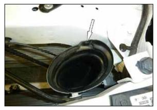
7. Remove the plastic retaining clip that secures the fresh air intake duct to the core support, then pull the duct forward to disengage it from the factory air filter housing.
