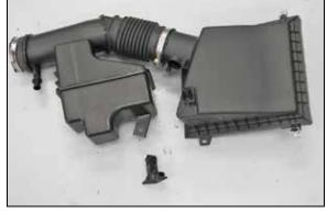
15. Remove the mass air sensor from the factory air filter housing.
