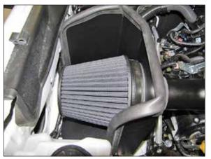
11. Install the provided edge trim onto the K&N<sup>®</sup> heat shield as shown.
