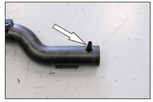
17. Install the provided NPT vent fitting into the  $K\&N^{\circledast}$  intake tube as shown.
