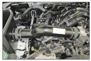
18. Install the intake tube into the coupling hose at the throttle body and then into the coupling at the filter adapter. Adjust the tube for best fit and then secure with the provided hose clamps.
