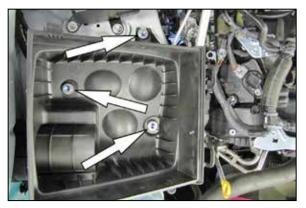
7. Remove the three bolts securing the lower air filter housing to the inner fender and then remove the lower air filter housing from the vehicle. **NOTE: K&N Engineering, Inc., recommends that customers do not discard factory air intake.**
