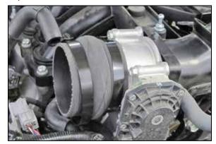
13. Install the provided hump coupler (08171) onto the throttle body and secure with the provided hose clamp.
