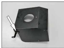
9. Install the provided heat shield bracket (07958) onto the  $K\&N^{\otimes}$  heat shield as shown.
