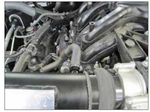
19. Connect the crank case vent fitting onto the vent fitting installed into the  $K\&N^{\otimes}$  intake tube.
