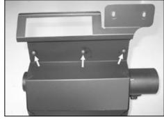
22. Install the three supplied rubber bumpers into the three holes in the heat shield from the bottom up.
