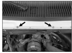
27. Place the two supplied spacers onto the cowl assembly at the air box mounting location as shown.
