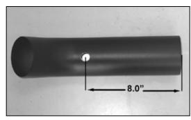
25a. On vehicles equipped with an external temperature sensor; measure and mark the tube 8.0" (from the straight end of the tube, on the inside radius of the bend). Then, drill a 5/8" ID hole in the tube as shown
