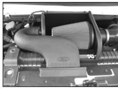
32. Install the factory fresh air scoop onto the heat shield and then latch it into the cut out and factory opening as shown.
