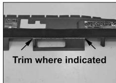
31a. On vehicles that the cowl cover conceals the air box mounting bolts, trim the cover as indicated by the dashed line so that the cover will sit flat onto the cowl.
