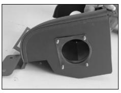
20. Install the remaining mass air sensor gasket onto the studs of the filter adapter protruding through the heat shield.
