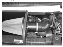
29. Insert the K&N® intake tube into the silicone hose at the throttle body and secure with the provided hose clamp.
