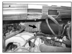
7. Loosen the hose clamp that secures the stock intake tube to the bellows at the throttle body.
