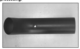
25b. Install the provided grommet into the hole drilled into the intake tube (during the previous step) as shown. Then, install the air temperature sensor into the grommet.
