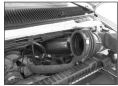
8. Remove the intake tube from the vehicle. NOTE: K&N Engineering, Inc., recommends that customers do not discard factory air intake.
