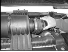
4. Loosen the hose clamp that secures the intake tube to the air filter housing and then disconnect the intake tube from the air filter.
