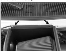
30. Using the factory bolts removed in step #3, secure the heat shield to the cowl.
