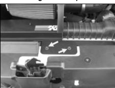
31. Using the factory bolts removed in step #5 secure the heat shield to the radiator core support.
