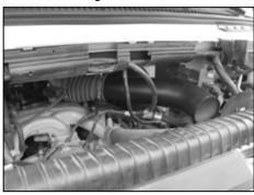
26. Install the K&N® intake tube into the bellows at the throttle body and secure with the factory hose clamp.
