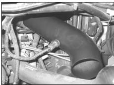
26a. On vehicles equipped with an external air temperature sensor; re-connect the air temperature sensor electrical connection as shown.
