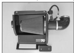
25. Reconnect the mass air sensor primary connector as shown.
