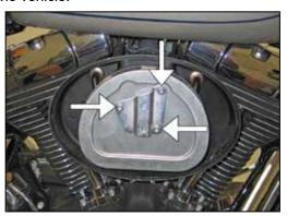
3. Remove the three bolts that secure the air filter to the filter base and then remove the air filter along with the crankcase breather tubes.
