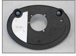
7. On models equipped with an EVAP vent line, cut out the provided template and place it on the filter base plate as shown. Mark the base plate for the ½"ID drill hole.
