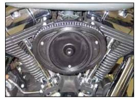
14. Install the air filter onto the base plate and secure with the provided three bolts.
