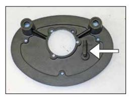
8. On models equipped with an EVAP vent line, drill a ½"id hole in the base plate at the location marked in step #7. Then install the provided grommet and 90° hose mender as shown.
