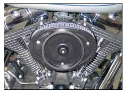
14. Install the air filter onto the base plate and secure with the three bolts provided.NOTE: Apply one drop of thread locker to each
