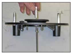
10. Install the three provided spacers onto the base plate as shown.
