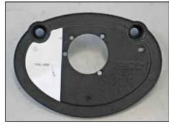
7. On models equipped with an EVAP vent line, cut out the provided template and place it on the filter base plate as shown. Mark the base plate for drilling a ½"ID hole.
