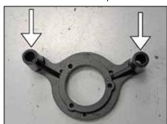
8. Install two of the provided O-rings into the crankcase breather plate as shown.
