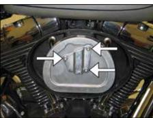
3. Remove the three bolts which secure the air filter to the filter base and then remove the air filter along with the crankcase breather tubes.
