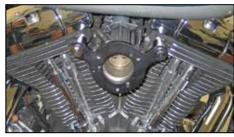
9. Install the crankcase breather plate along with the two remaining o-rings, mounting bolts (with one drop of thread locker) and throttle body gasket as shown.
