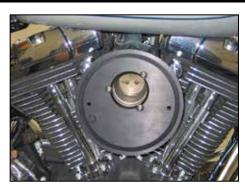
10. Install the three filter base plate mounting bolts into the base plate; install the remaining gasket and one drop of thread locker on each bolt. Secure the filter base plate to the breather plate as shown.
