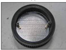
12. Install the K&N® air filter onto the top plate as shown.
