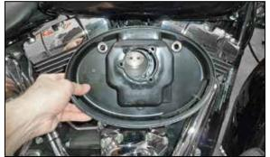
6. Remove the air filter breather base as shown. NOTE: K&N Engineering, Inc. recommends that customers do not discard the factory air intake components.
