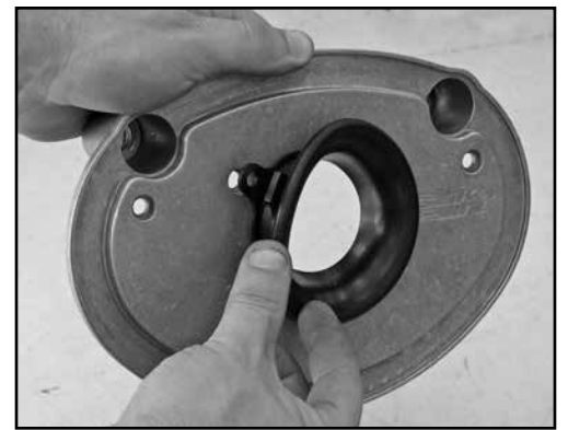
7. Install the velocity stack onto the supplied back plate.
