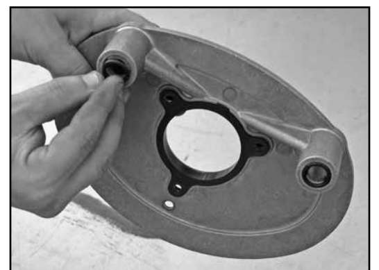
9. Install the two o-rings into the back plate standoffs.
