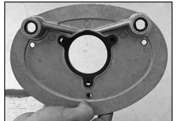
8. Align the holes on the velocity stack with the bolt holes in the back plate.
