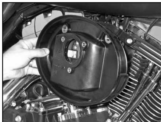
5. Remove the stock back plate.
