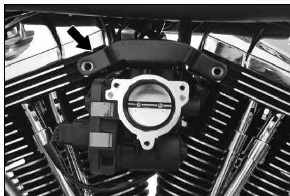
6. Do not remove the throttle body support bracket.
