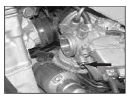
9. Locate fuel mixture screw and turn screw clockwise until lightly seated. Now turn screw counterclockwise 2-1/2 turns.
