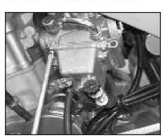
Loosen the four screws on the float bowl. NOTE: The float bowl may still contain fuel.
